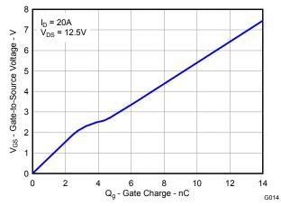
Figure 14. Control MOSFET Gate Charge
