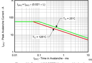
Figure 26. Control MOSFET Unclamped Inductive Switching
