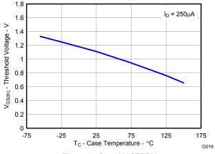
Figure 19. Sync MOSFET V<sub>GS(th)</sub>
