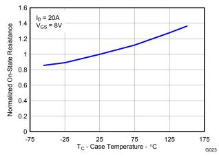
Figure 23. Sync MOSFET Normalized R<sub>DS(on)</sub>
