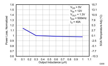
Figure 9. Normalized Power Loss vs. Output Inductance
