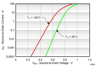
Figure 24. Control MOSFET Body Diode
