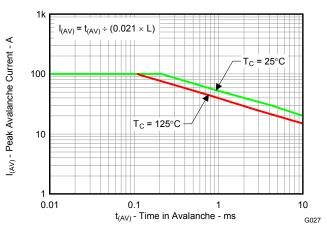
Figure 27. Sync MOSFET Unclamped Inductive Switching
