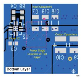
Figure 30. Recommended PCB Layout (Top Down View)
