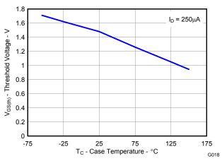
Figure 18. Control MOSFET V<sub>GS(th)</sub>
