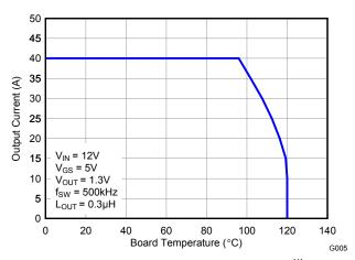
Figure 5. Typical Safe Operating Area<sup>(1)</sup>
