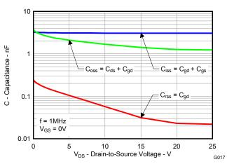
Figure 17. Sync MOSFET Capacitance
