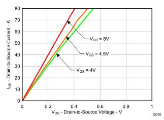
Figure 10. Control MOSFET Saturation
