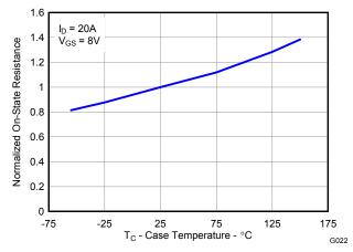
Figure 22. Control MOSFET Normalized R<sub>DS(on)</sub>
