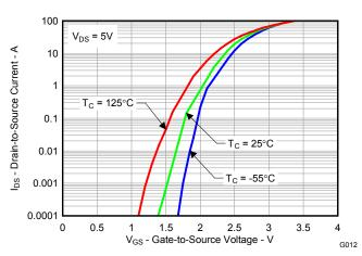
Figure 12. Control MOSFET Transfer
