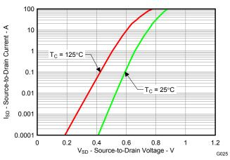
Figure 25. Sync MOSFET Body Diode
