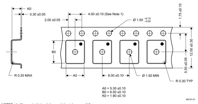
NOTES: 1. 10-sprocket hole-pitch cumulative tolerance ±0.2
