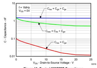
Figure 16. Control MOSFET Capacitance
