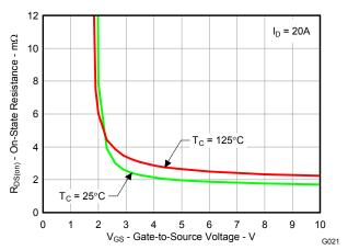
Figure 21. Sync MOSFET  $R_{DS(on)}$  vs  $V_{GS}$
