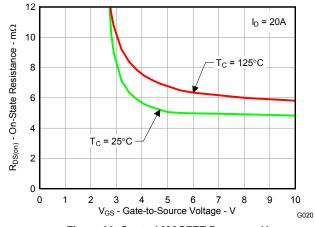
Figure 20. Control MOSFET  $R_{DS(on)}$  vs  $V_{GS}$
