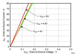
Figure 11. Sync MOSFET Saturation
