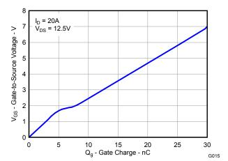
Figure 15. Sync MOSFET Gate Charge
