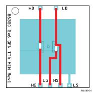
Max  $R_{\theta JA} = 50^{\circ} C/W$  when mounted on 1 inch² (6.45 cm²) of 2-oz. (0.071-mm thick) Cu.
