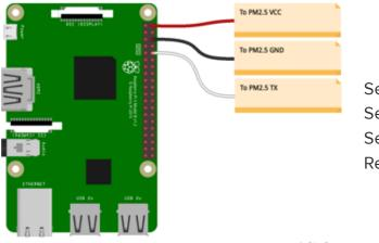
Here's an example using the Pi's built-in UART:
