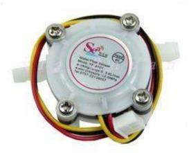
Water flow sensor consists of a PVC body, a water rotor, and a hall-effect sensor. When water flows through the rotor, rotor rolls. Its speed changes with different rate of flow. The hall-effect sensor outputs the corresponding pulse signal. This one is suitable to detect flow in water dispenser or coffee machine.
