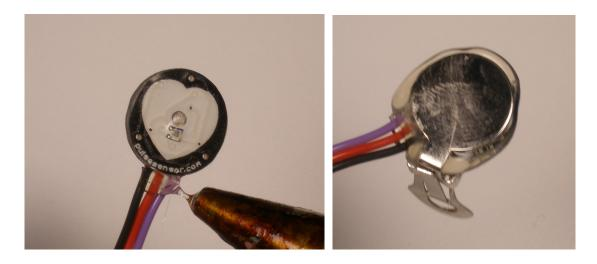
Allow the hot glue to ooze out around the ear clip. That will ensure good coverage. Take care not to let the hot glue cover around the ear clip hinge, as that could get in the way of it working. Trimming is easy with nail clippers (as above) or your trimming tool of choice. Don't trim the wires by mistake!!!
