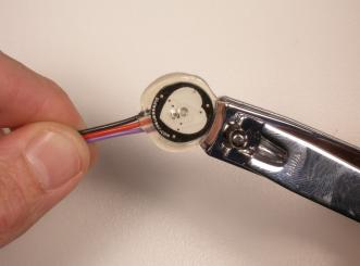
Once the hot glue has cooled (wait for it!) the blue tape will peel off very easily. Check your work to make sure that there are not exposed electrical connections! Next is trimming. I find the easiest way is to use nail clippers. Flush cutting wire snips work too. Take care not to clip the wires!!! And leave enough around the cable to act as a good strain-relief
