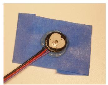
Then, while the glue is still very hot, press the Pulse Sensor glue-side-down onto the sticky side of a piece of blue tape (I believe that blue tape has magical properties, but if you don't have blue tape other kinds of tape will work just as well).
