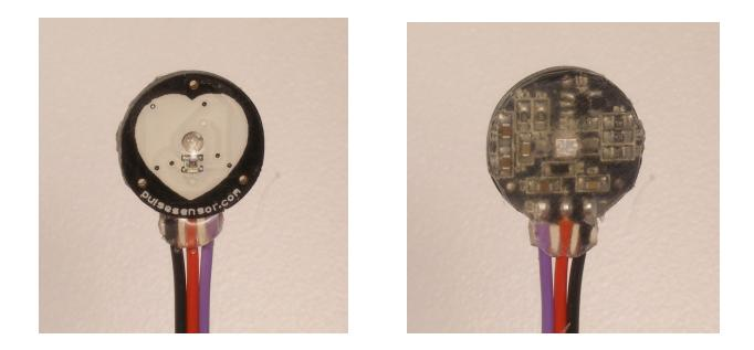
This is the basic Pulse Sensor Hot Glue Seal, It's also got the clear vinyl sticker on the front face. We're calling this 'Water Resistant', ready to be handled and passed around from fingers to earlobes or whatever. It is not advised to submerge or soak the Pulse Sensor with this basic seal.
