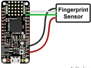
Board GND to sensor GND (black wire)
