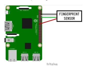
Pi GND to sensor GND (black wire)
