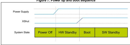
Figure 7. Power up and boot sequence
