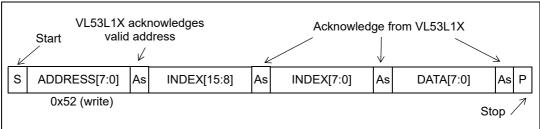
As data are received by the slave, they are written bit-by-bit to a serial/parallel register. After each data byte has been received by the slave, an acknowledge is generated, the data are then stored in the internal register addressed by the current index.
