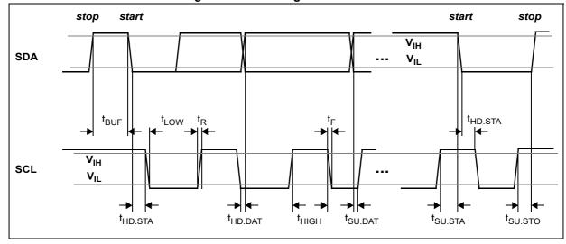
Figure 17. I<sup>2</sup>C timing characteristics
