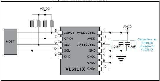
Note: Capacitors on external supply AVDD should be placed as close as possible to the
