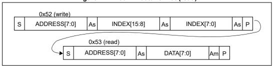
At the end of each byte, in both read and write message sequences, an acknowledge is issued by the receiving device (that is, the VL53L1X for a write and the host for a read).
