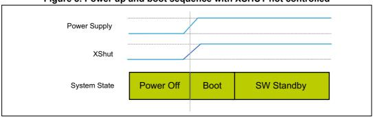
Figure 8. Power up and boot sequence with XSHUT not controlled
