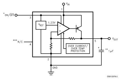
$*ON/\overline{OFF}$  input must be actively terminated. Tie to  $V_{IN}$  if this function is not to be used.
