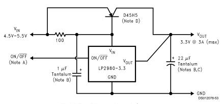
FIGURE 7. 5V to 3.3V @ 3A Converter
