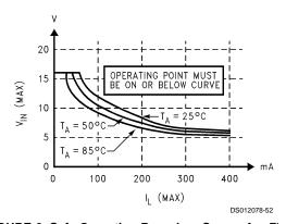
FIGURE 6. Safe Operation Boundary Curves for Figure 5
