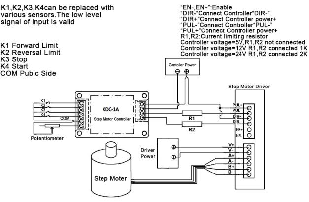
If the voltage of driver power is less than 32V,the controller and driver can share a single power supply.
